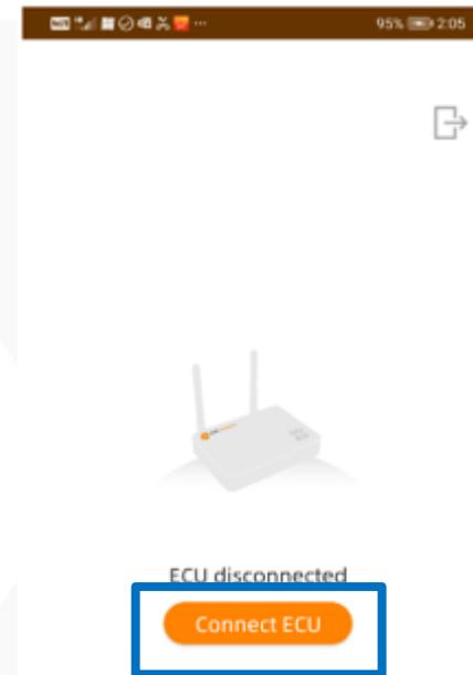
Warning: if your ECU gets a button "AP" on the side of the casing, the Wi-Fi hotspot is activated for 1 hour after the ECU is powered.
